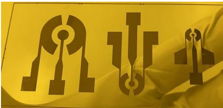
Gold electrodes with dimensions of 4mm, 2mm and 1mm fabricated using photolithography technique
