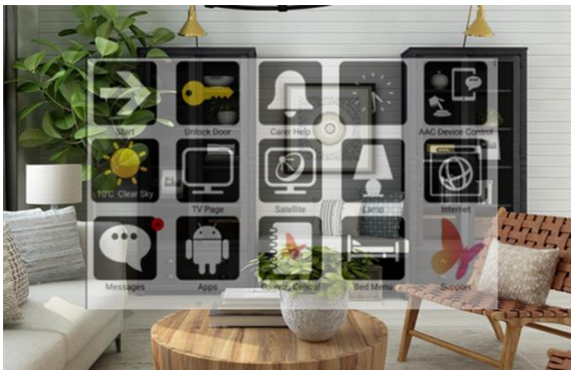
Figure 1: A mock up of how the smart glasses display would appear for the user.
