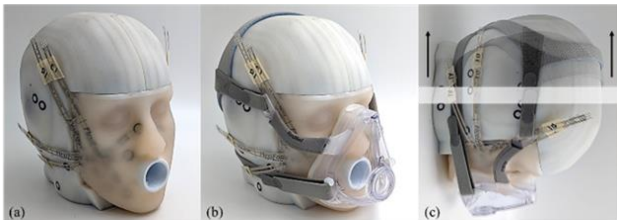
(a) head phantom with embedded pressure sensors visible; (b) phantom with ResMed mask attached; (c) orientation of phantom during experiment.
